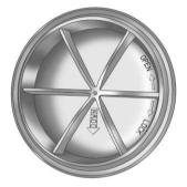
From the back side of the headlamp assembly, remove the top cap to replace the low-beam headlamp/DRL bulb.
